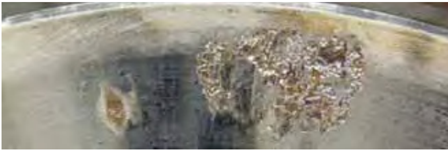
Figure 1: Damage caused by bearing failure
